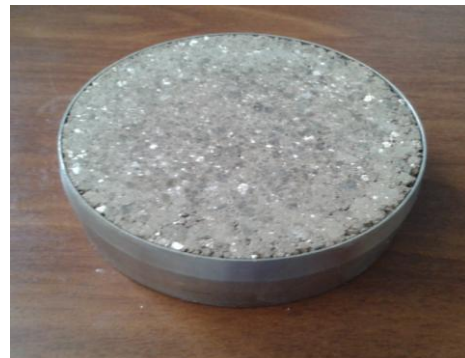
Fig. 4 Soil sample after the first of wet-dry cycle
